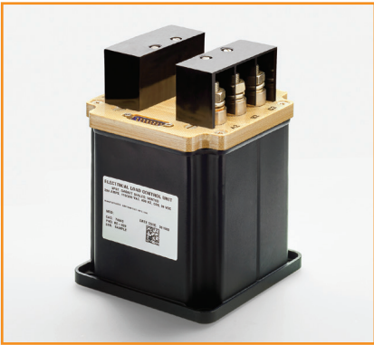
Electrical load control units (ELCUs) provide I 2 T, differential, phase imbalance, and over/under voltage and frequency protection.
